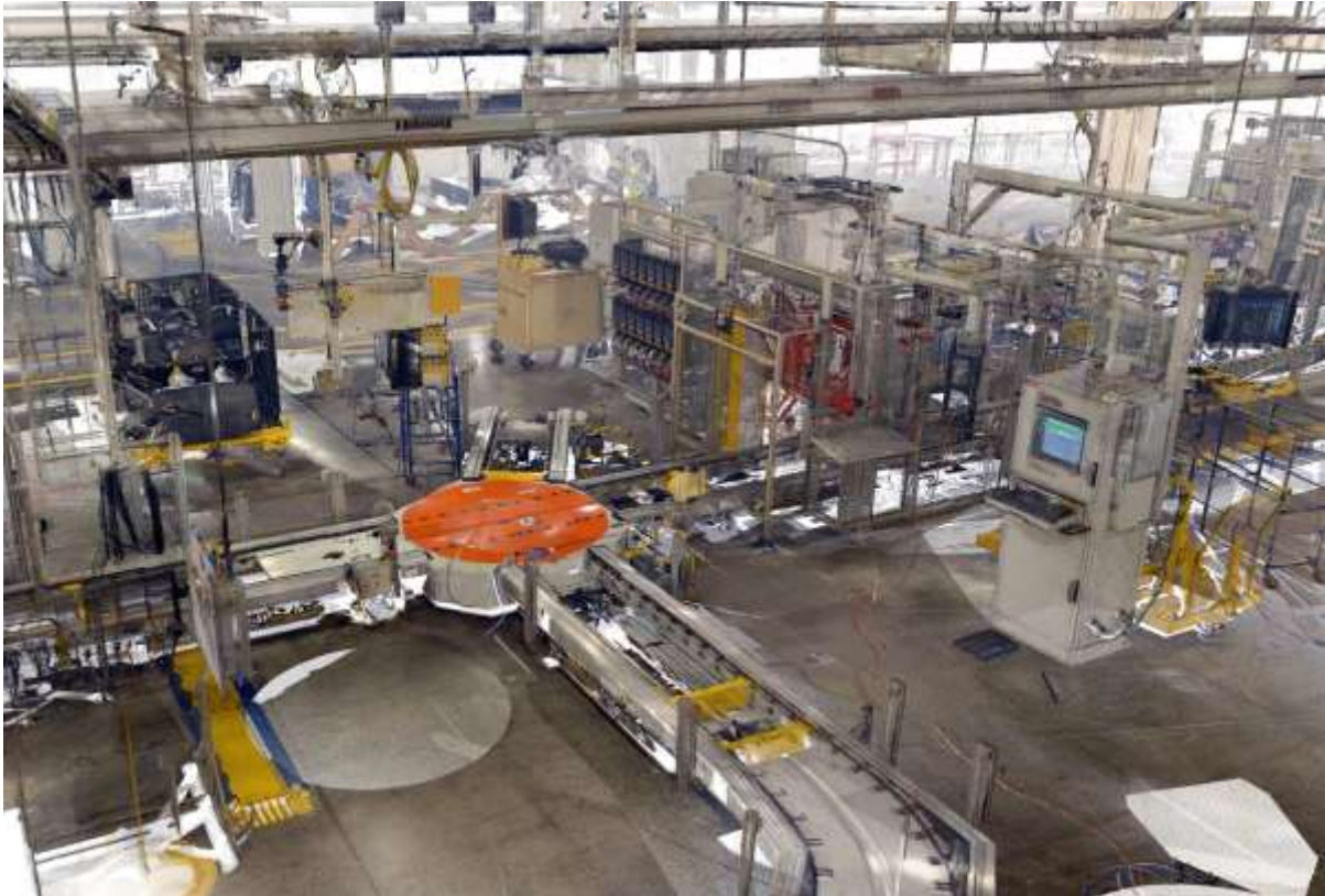
3D point cloud model (~4.5 billion points) of a Ford motor car plant in the USA – captured by a FARO Photon 120 scanner.
